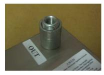
Step 2. Spray a small of lubricant in the Outlet side of the valve.
